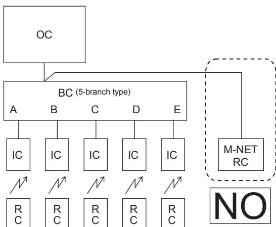
3-1. Plural indoor units cannot be operated by a single remote controller.
