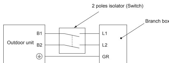
Be sure to connect the outdoor-branch box/indoor-branch box connecting cables directly to the units (no intermediate connections). Intermediate connections can lead to communication errors if water enters the cables and causes insufficient insulation to ground or a poor electrical contact at the intermediate connection point. (If an intermediate connection is necessary, be sure to take measures to prevent water from entering the cables.)
